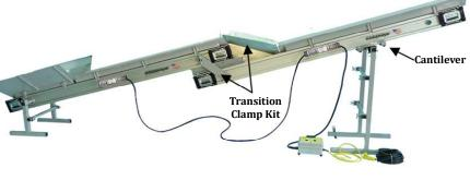
A cantilever set on a leg kit enables the discharge conveyor to overhang.
