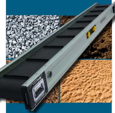
Modular construction lends itself to a customer designed installation. Units can be locked together using a clamp kit and 4 modules can provide a 40 ft. (12m) unsupported span. Use the 20 ft kit and 2 units become a solid 20 ft (6m) unit. There are hoppers for hand loading and hoppers for machine loading. For greater tonnage, run units in tandem with a doublewide hopper. Side extensions can reduce spillage. Wheels are also available.
